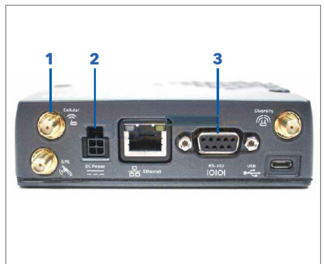
Figure 19: Attach the antenna cable to point 1 on the modem
