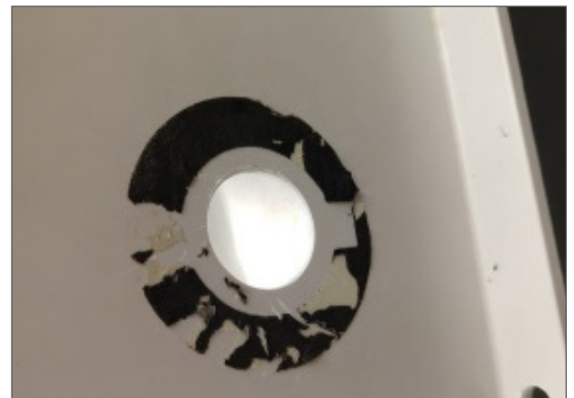
Figure 7: Showing portion of gasket still attached to the enclosure
