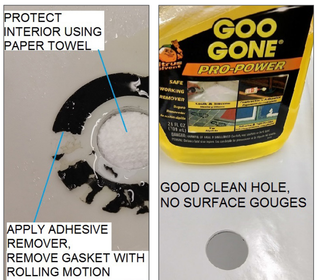
Figure 10: Remove the remains of the old antenna gasket
