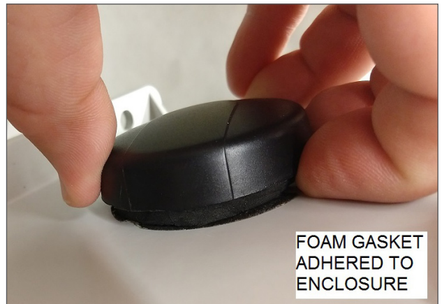
Figure 6: Showing the foam gasket adhered to the enclosure
