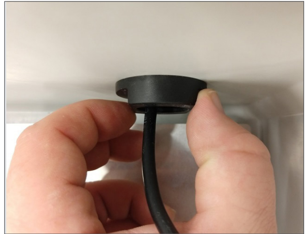
Figure 5: Remove the antenna connector
