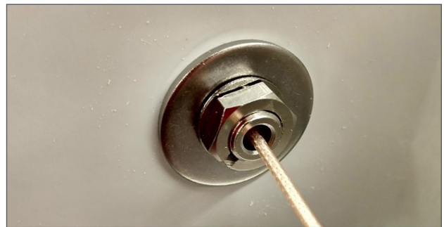
Figure 12: Secure the antenna to the enclosure
