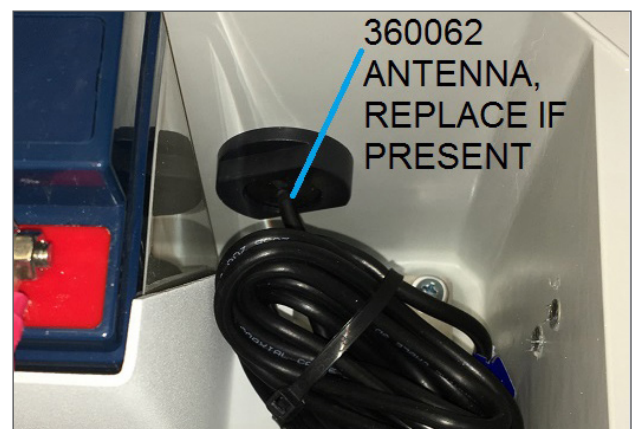
Figure 4: Replace the 360062 black puck antenna with the antenna provided in the 203228 kit
