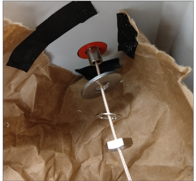
Figure 11: Install the new antenna
